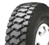
**DMO4****Drive axle tyre for off road with excellent traction & durability**
